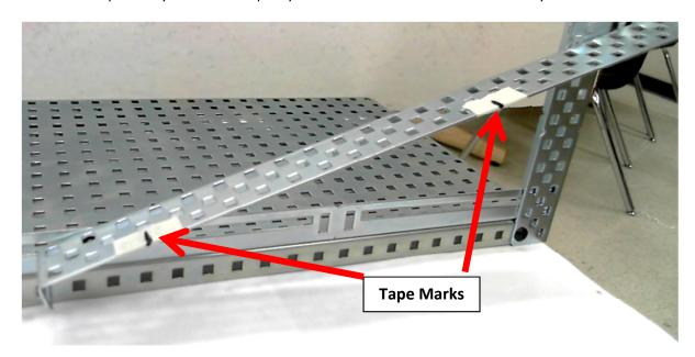
2. Measure the length of the inclined plane (L) between the two points and record it on your data sheet.
