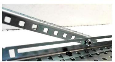
5. Gather parts and assemble pulley that will be attached at the top of the inclined plane. Parts—2" drive shaft, 3 shaft collars, 1 plus gusset, 2 thin spacers, 5/64 wrench for adjusting set screws in shaft collar.
