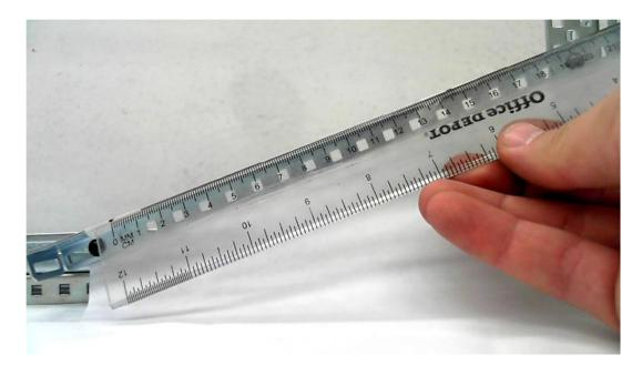
3. Measure the height from the table to the lower point and record it. Then measure the height from the table to the upper point and record it. Subtract these two measurements to find the height of the inclined plane between the two points (H) and record it on your data sheet.
