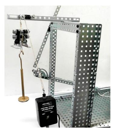
Example of Moveable Pulley Set-up and Effort Force Measurement
